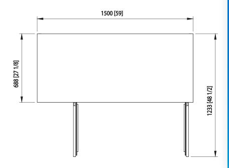
2 Door Capacity 19.4 Cu.Ft. Shelves Refrigerant R-290 Temperature 33°F ~ 39°F Range Sliding Easy Maintenance Condensing Unit 9.8 ft long (3m) flexible three Connection wire cord with modeled plug HP 3/8 Voltage 115V/60Hz **Amps** 3.8 NEMA Config. NEMA 5-15 Lighting Interior LED lighting
