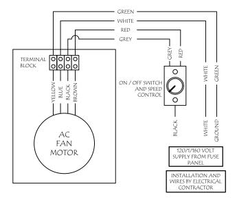
VARIABLE SPEED CONTROL DIAGRAM NOT TO SCALE
